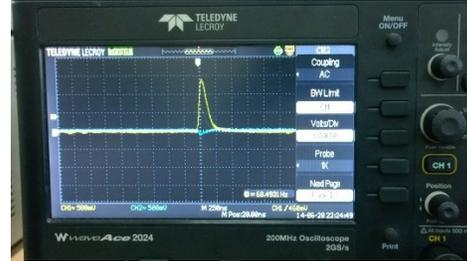
**Figure 16:** Input (blue) and output (yellow) pulses from the Mk. I SiPM and the Mk. II amplifier.
