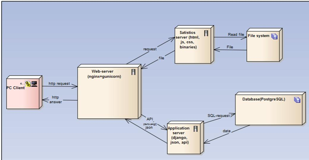
Fig. 1 High-level of OCAM architecture (UML)
