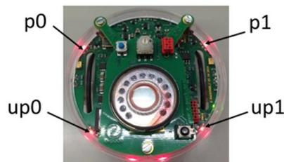
Figure 2: Layout and meanings of the LEDs on the small robot
