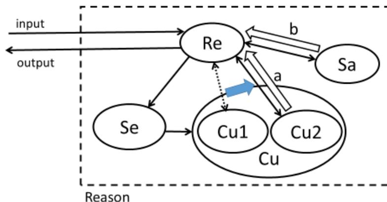
Figure 4: Reason subsystem when curiosity has grown adequately, a safe environment is secured, and an unknown area is located immediately in front of the robot
